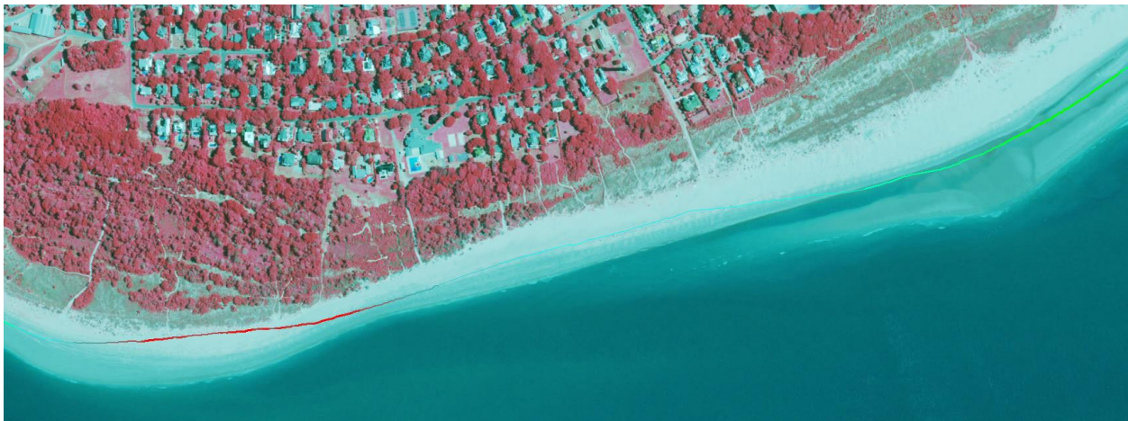
Figure 12. Recent shoreline colored by change significance on 2019 CIR (NAIP) imagery. Red parts of the shoreline indicates significant erosion, green significant accretion, and blue a location with no significant variation from the historic trends.
