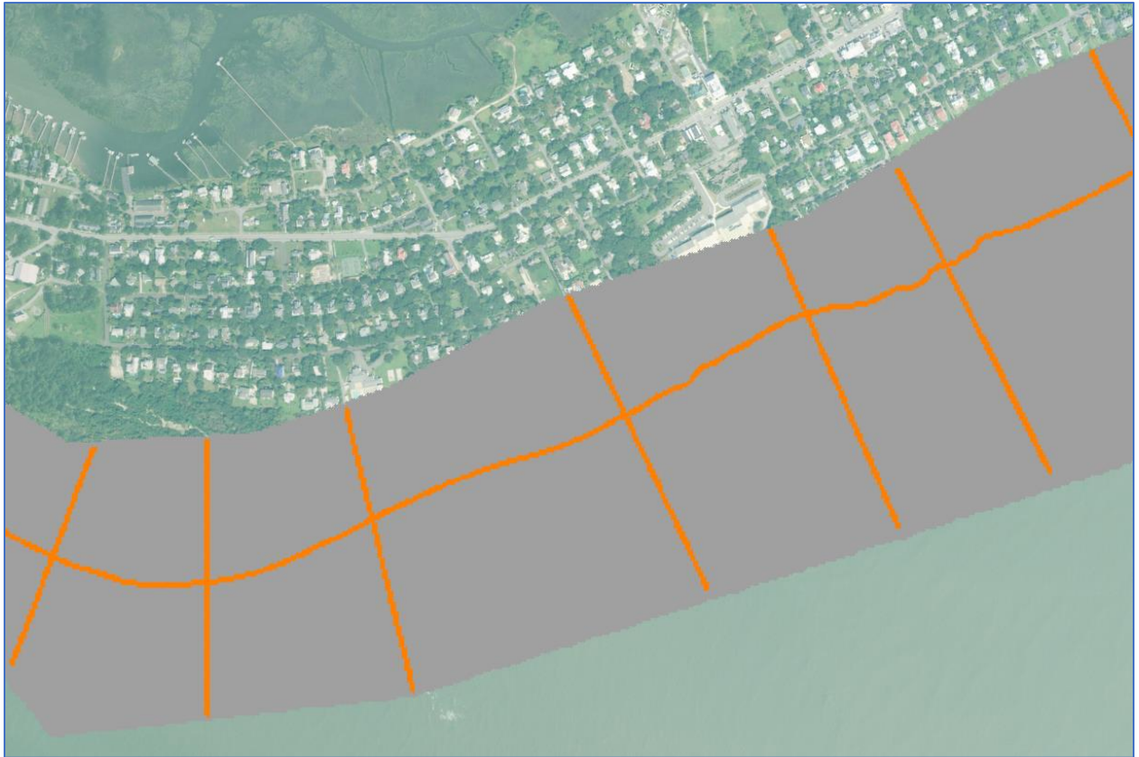
Figure 5. MBT surface converted to lidar points. Points falling on the profiles and shorelines were classified differently than the surrounding points.
