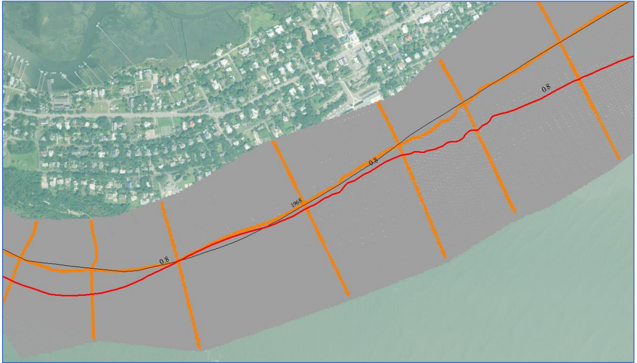
Figure 6. '1968 synthetic lidar points' with the 1968 shoreline (black line) and the MBT shoreline (red)
